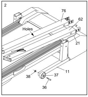
3. Insert a Plastic Shim (97) into each side of the post on the right side of the Base (11). Next, orient the Right Upright (62) as shown, and insert it into the Base. Make sure that the Wire Harness (21) does not fall into the Right Upright. Be careful to avoid pinching the Wire Harness. Note: If necessary, tap the Right Upright with a rubber mallet until it is fully seated in the Base. If the Right Upright cannot be fully seated, remove the outer Plastic Shim and then insert the Right Upright.
